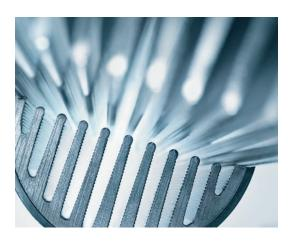
The **aluFer® heat exchanger** made from a combination of aluminium (on the inside) and stainless steel (on the outside) provides maximum conductivity. Due to its vertical installation in the boiler, the temperature stratification of the heating water is supported, contributing to an additional increase in efficiency. The modern gas condensing technology uses fuel up to 15% more efficiently than a low-temperature boiler.
