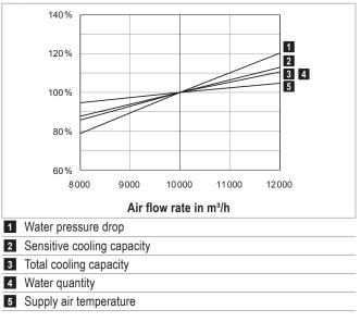
Fig. B5: Changes in output data depending on the air flow rate
