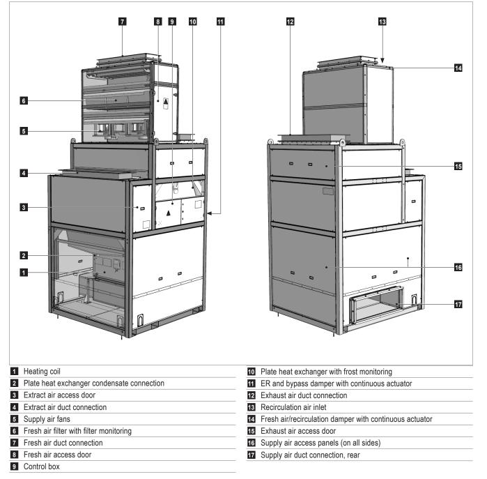
Fig. A2: Unit construction
