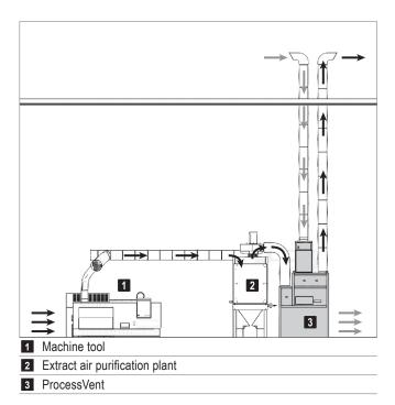
Fig. C1: The ProcessVent unit forms one overall system with the extract air purification plant.
