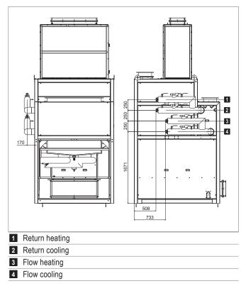
Fig. D9: Dimensional drawing for 4-pipe switching (dimensions in mm)
