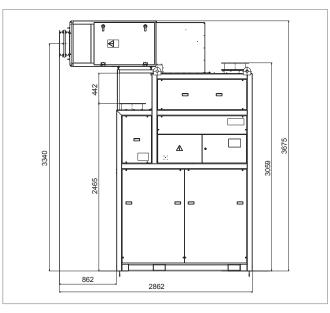
Fig. D5: Dimensional drawing for fresh air module, horizontal (dimensions in mm)
