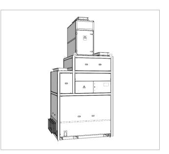
Fig. D1: Unit with supply air duct connection, left
