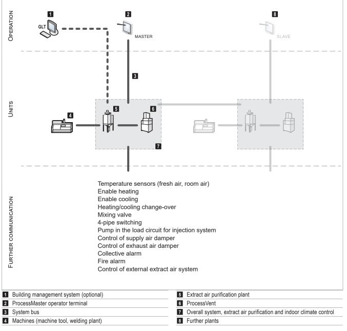
Fig. G1: ProcessNet system set-up
