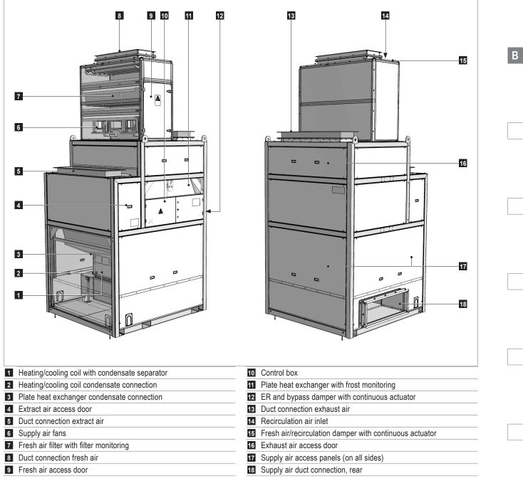
Fig. B2: Unit construction
