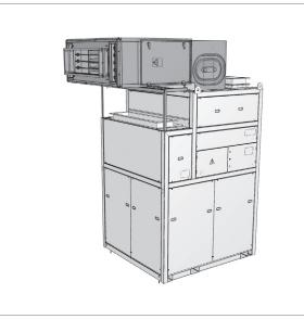
Fig. D4: Unit with fresh air module installed horizontally
