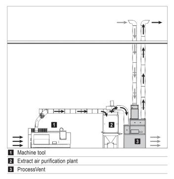
Fig. A1: The ProcessVent unit forms one overall system with the extract air purification plant.
