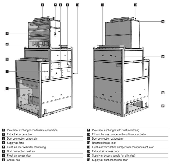
Fig. C2: Unit construction
