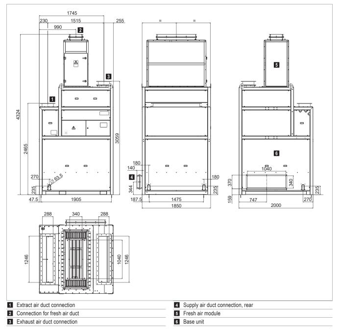
Fig. C5: Dimensional drawing (dimensions in mm)
