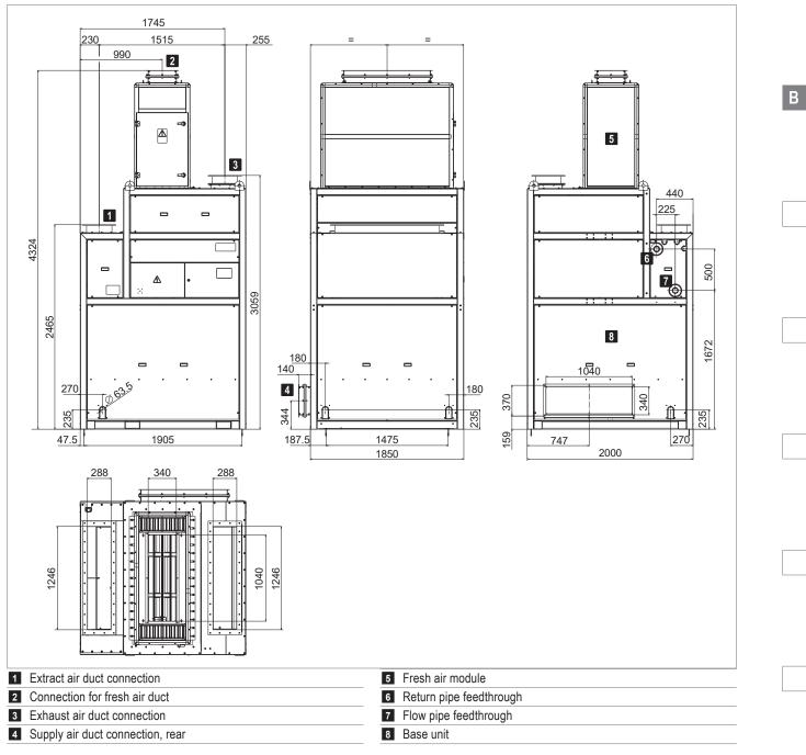
Fig. B6: Dimensional drawing (dimensions in mm)
