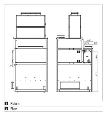
Fig. D7: Dimensional drawing for hydraulic connections (dimensions in mm)
