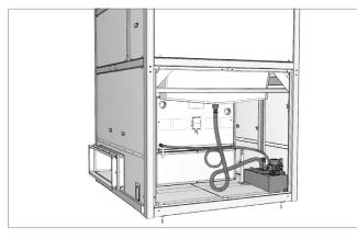
Fig. D11: Return pump station installed in the unit
