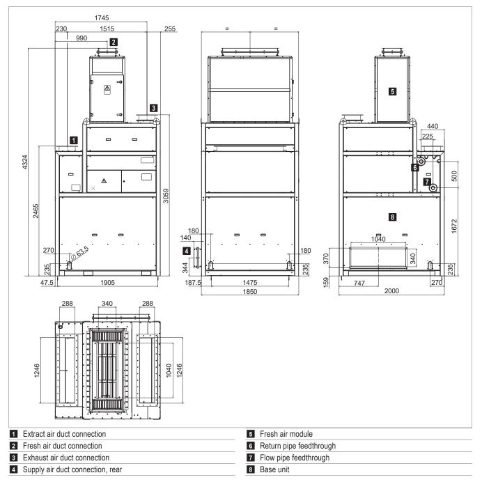
Fig. A5: Dimensional drawing (dimensions in mm)
