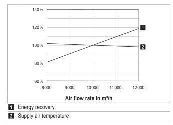
Fig. C4: Changes in output data depending on the air flow rate
