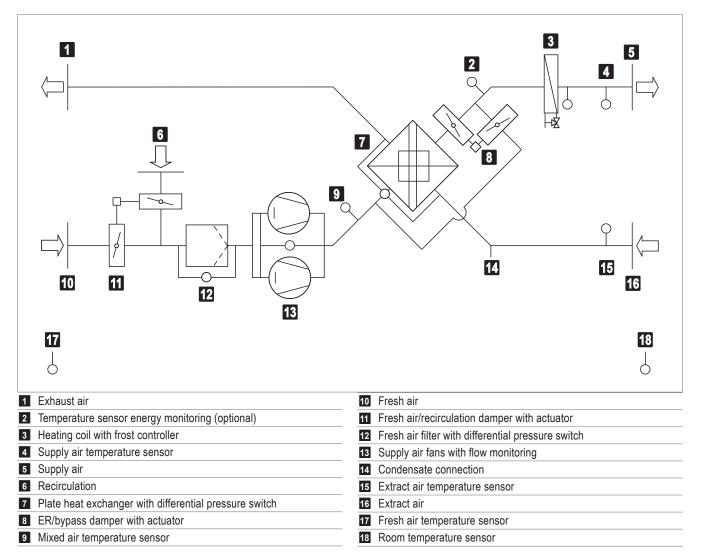
Fig. A3: Function diagram
