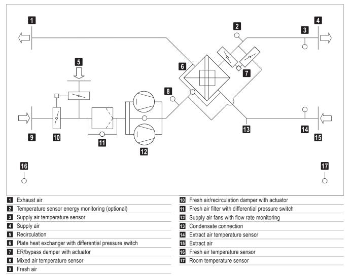
Fig. C3: Function diagram
